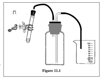
3. Before heat is applied to the test tube, the assembly must be checked to make sure that water will not be transferred from the bottle to the beaker by siphoning. Proceed with this checkthas stopper that me proceeding. If there is no evidence of siphoning, proceed to the proceeding.
